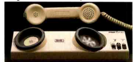
Here's the 2nd included Modem. It's an external Acoustic Modem. One last word about modems. If you're Next Page Please. . .
