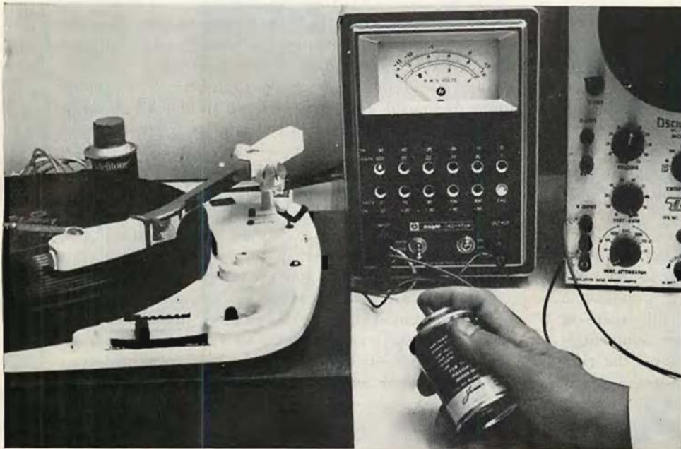
Treble attenuation test revealed no impairment of high frequency response by anti-static liquids. High frequency output from test record was checked on VTVM before and after application of fluids. Waveform monitored on oscilloscope also remained unaffected by the anti-static treatment.
