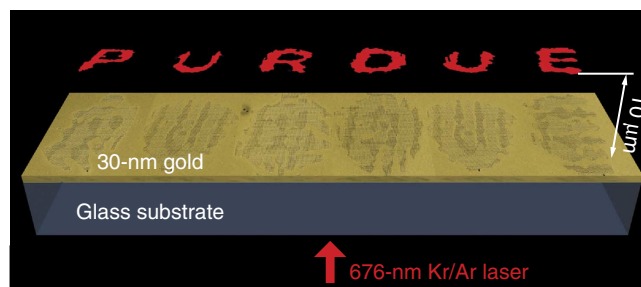
Figure 3 | Holographic images produced by the experimental metasurface holograms. The image is of the word ‘PURDUE’. The sample is illuminated by a Kr/Ar laser at 676 \text{ nm} from the glass substrate side. The images are obtained experimentally at a plane 10 \mu\text{m} above the metasurface hologram. The patterns on the gold film are the FE SEM images of the fabricated samples.
