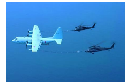
Transport aircraft with aerial refueling function (KC-130H) / rescue helicopters (UH-60J)
