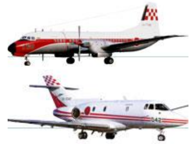
Flight check aircraft (the pictured aircraft are existing ones) (above: YS-11FC; below: U-125)
