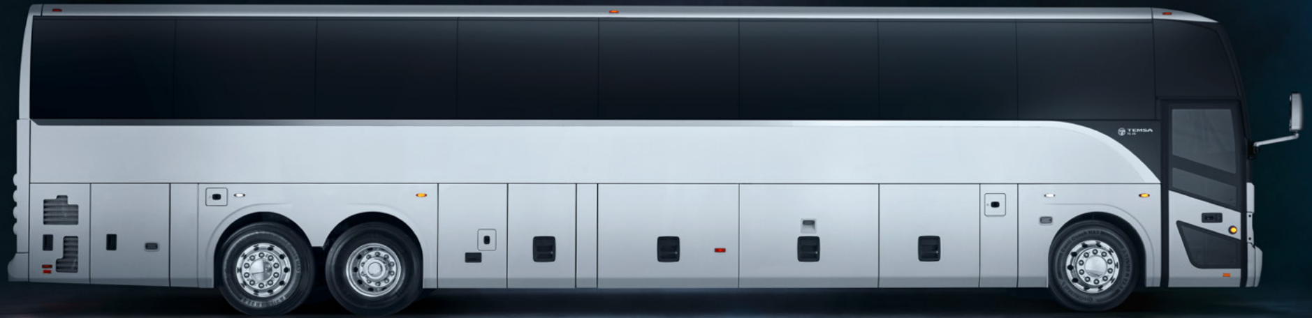
Double-glazed side windows providing air conditioning, safety and noise isolation
