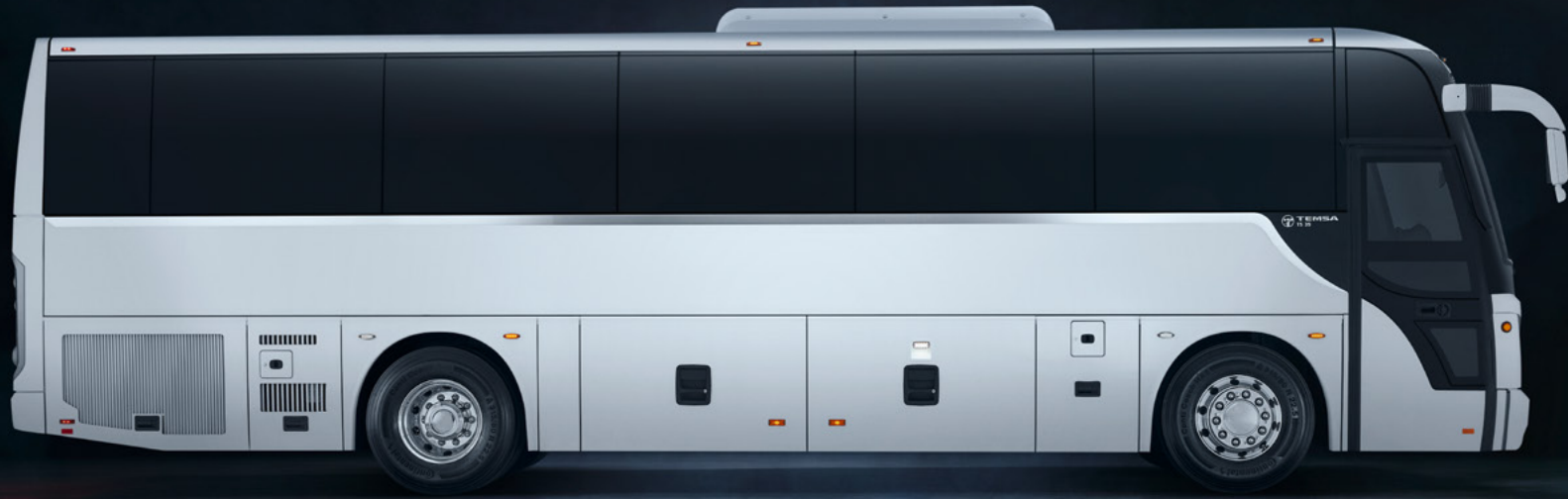
Double-glazed side windows provide air conditioning, safety, and noise isolation
