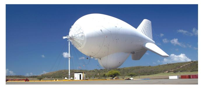
U.S. Customs and Border Protection's Air and Marine Operations (AMO) uses the Tethered Aerostat Radar System (TARS) to provide long-range detection of low-altitude aircraft at the radar's maximum range. The elevated sensor mitigates curvature of the earth and terrain masking limitations.
