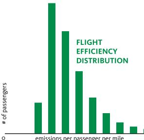
Taken together, diversity in distance, aircraft, seating density, load factor, and freight share creates significant variation in overall emissions per passenger per mile. To reiterate, passenger carbon footprints per mile vary by more than a factor of ten across the industry, with many flights falling outside the peak of the bell curve.
