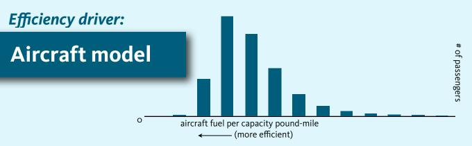
Like cars, planes vary in fuel efficiency. Engine technology, aerodynamics, size, and other factors affect the fuel required to haul a pound of cargo one mile. This variation is significant—an aircraft in the 90th percentile for efficiency uses less than half the fuel per capacity pound-mile as one in the 10th percentile (an aircraft's capacity pound-miles is the total quantity of weight it could carry multiplied by the flight distance).
