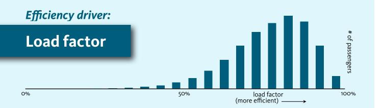
Passenger load factor—the portion of available seats filled on a given flight—has a major influence on each passenger's footprint, because total emissions are divided among the passengers on board. Fewer occupied seats means a larger share assigned to each person.
