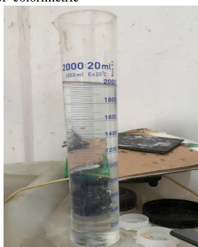
Figure 5. Measuring of settling velocity of the granules.
