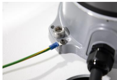
Figure 17: Grounding position for the robot
