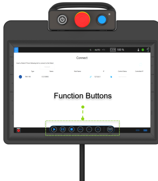
Figure 26: TM Teach Pendant (consisting of the TM Screen and Robot Stick)
