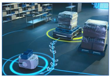
CAPS technology utilizes any compatible laser to detect a customizable target in the environment and enables the AMR to drive to the required location with unrivaled precision.
