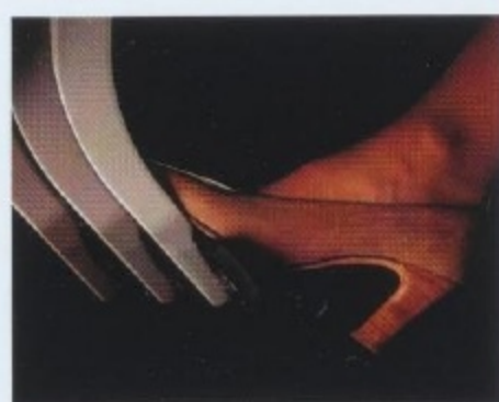
Adjustable power brake and accelerator pedals are available and can be electronically moved forward and back for your comfort. Positions can be set and recalled for two drivers, as part of the memory system.
