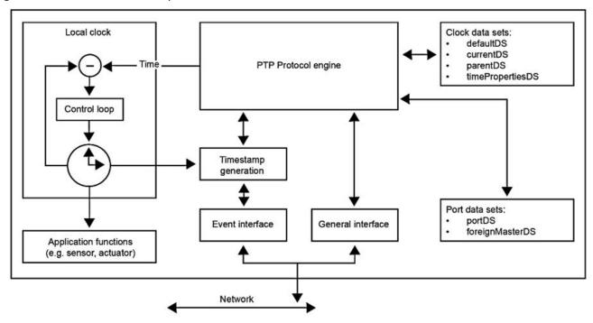
The ordinary clock executes the port state machine and *BMC* (Best Master Clock) algorithm to select the *PTP* port state. If the port is in the master state, the local clock is synchronized to an external source of time traceable to *TAI* (International Atomic Time) and *UTC* (Universal Coordinated Time) such as *GPS* (Global Positioning System) system. If the port is in slave state, the local clock is synchronized with its master clock.
