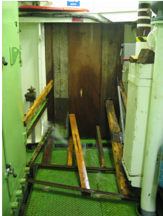
Figure SMO.3 Watertight door on Alliance during flooding (note water ingress).
