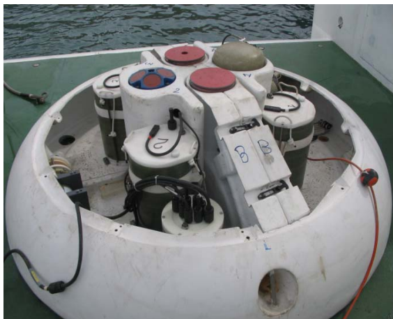
Figure ETD.1 Complete SEPTR unit without cover.
