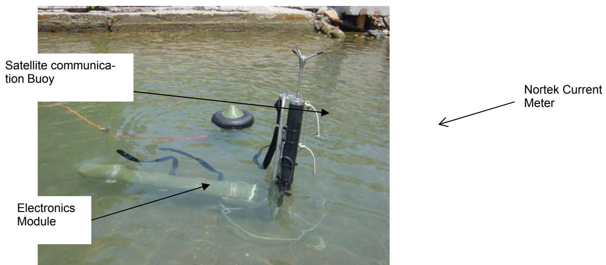
Figure ETD.3 Complete current meter showing three components of the system.
