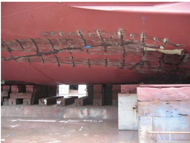
Figure SMO 4 NRV Alliance – underwater hull damage.
