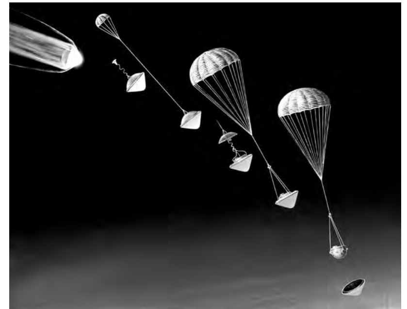
Figure 8.6. Atmospheric Probe parachute deployment sequence and separation of deceleration module components from descent module. After the high-speed entry phase during which the atmosphere slowed down the Probe's speed, a mortar deployed a small drogue parachute, the drogue chute opened, the aft cover of the deceleration module was released, the drogue parachute pulled the aft cover off and deployed the main parachute, and the forward heatshield was dropped. (NASA photo number AC89-0146-2)
