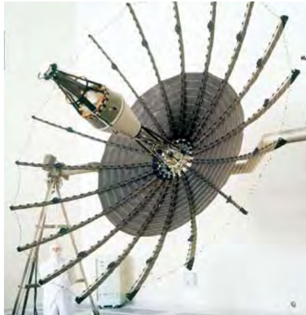
Figure 7.1. The unfurled high-gain antenna. (Adapted from JPL image number 230-893B)
