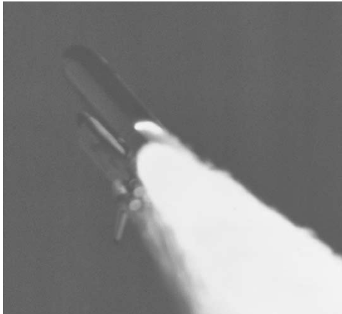
Figure 4.1. Booster rocket breach. At 58.778 seconds into powered flight, a large flame plume was seen just above the right-hand booster engine exhaust nozzle. (Johnson Space Center image number S87-25373, 28 January 1986)
