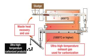
Next-generation sewage sludge carbonization system (ultra-high-temperature carbonizing furnace)
