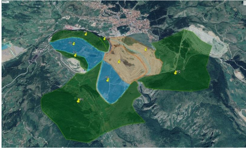
Figure 3 Positions of catchment areas in the wider area of the open pits Potrlica-Kalušiči after relocation of the Čehotina river (Google Earth satellite image)
