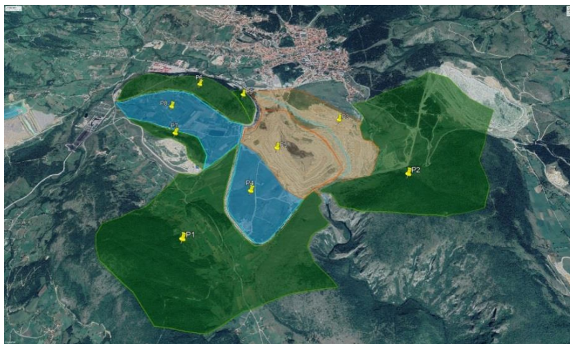
Figure 4 Positions of catchment areas in the wider area of the open pits Potrlica-Kalušiči after relocation of the Čehotina river (Google Earth satellite image)
