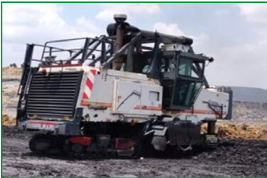
Surface Miner in operation at Sonepur Bazari Area of ECL
