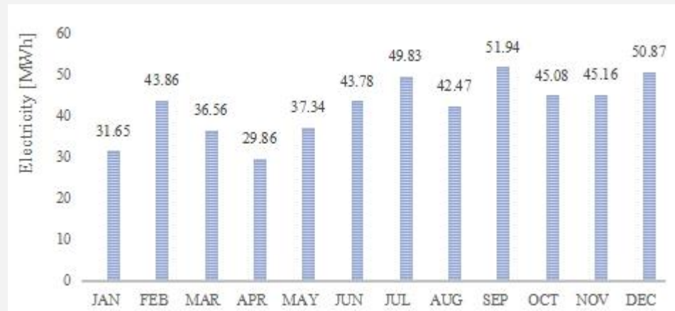
Figure 9. Electricity generation in a typical RoR Cuban SHP
