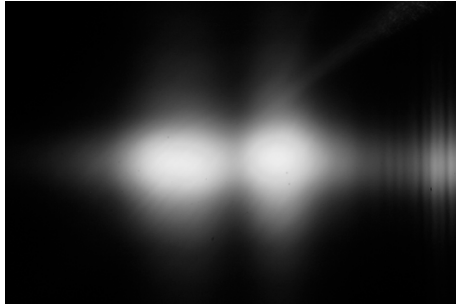
Figure 8.19: Image from XTM-90 with two-hole aperture with angle distance 20'
