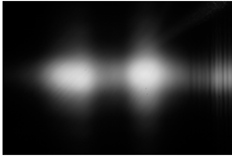
Figure 8.17: Image from XTM-90 with two-hole aperture with angle distance 30^\circ
