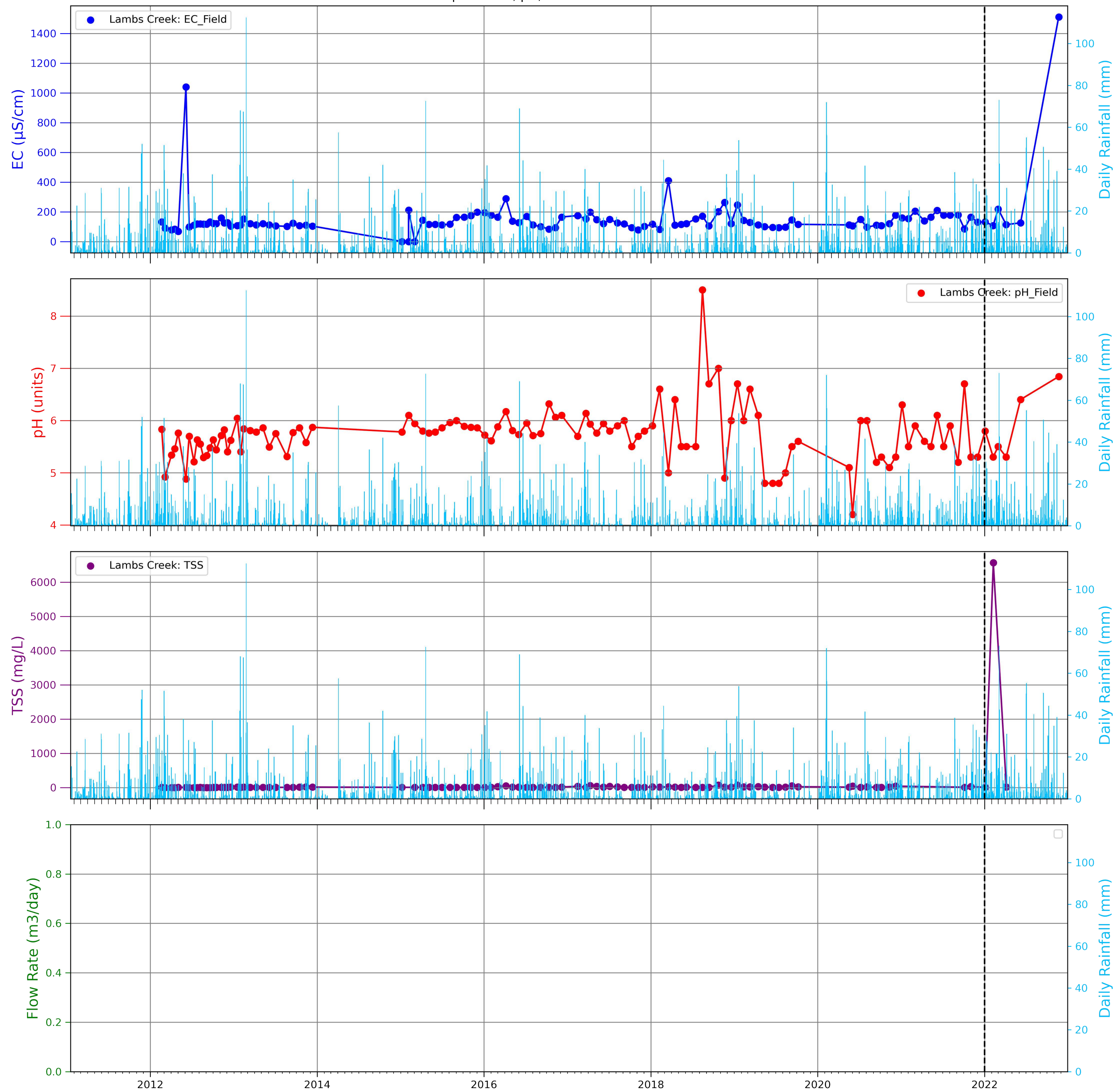
Time series plot of EC, pH, TSS and flow rate at: Lambs Creek
