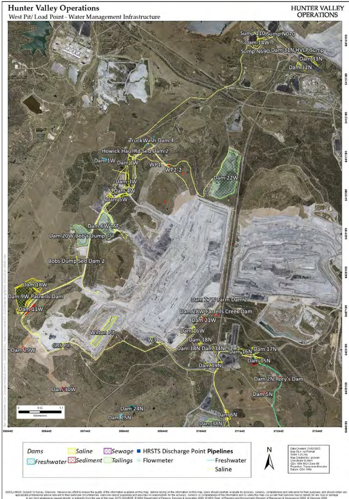
Figure 7-1: West Pit Water Management Infrastructure
