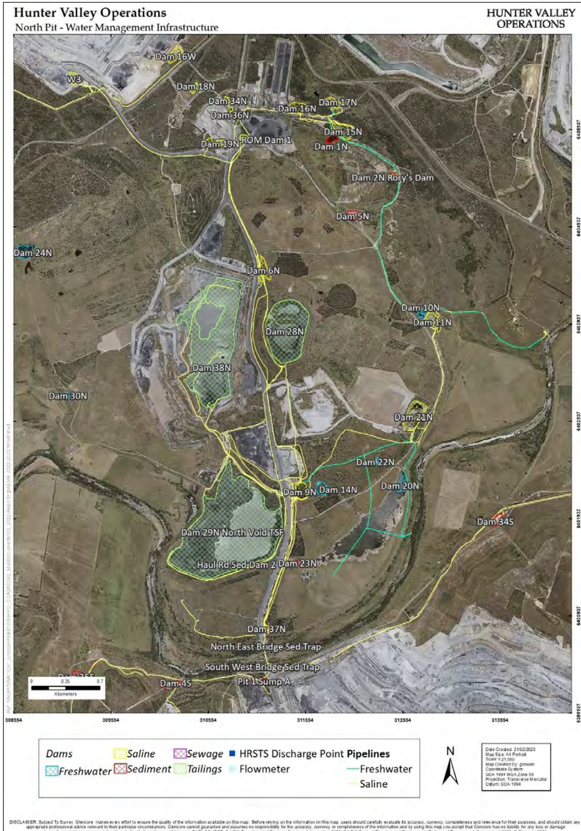
Figure 7-2: North Pit Water Management Infrastructure
