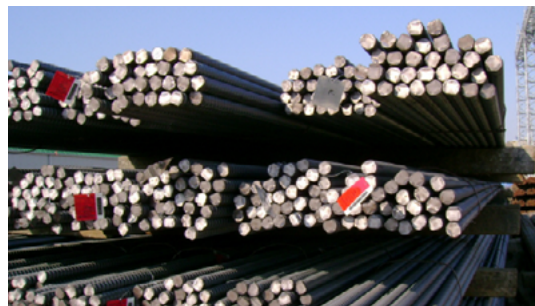
Rebar for nuclear power plant construction
