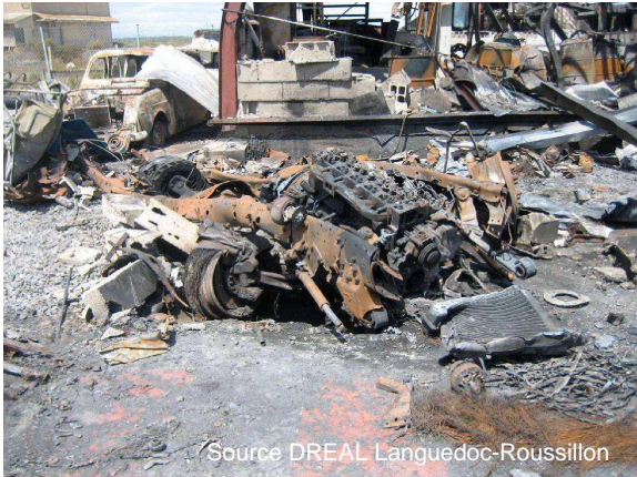
Wrecked tanker lorry after exposure to the BLEVE
