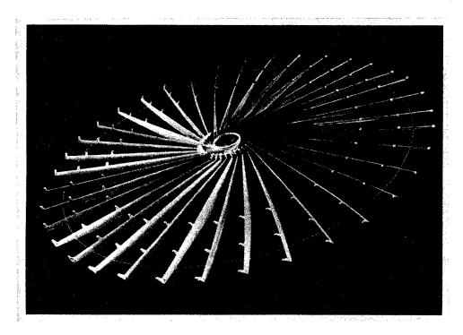
The Homing Overlay Experiment (HOE) used a warhead that expanded to destroy incoming warheads. In June 1984 it successfully intercepted a non-nuclear reentry vehicle. Credit: US Army Space and Strategic Defense Command
