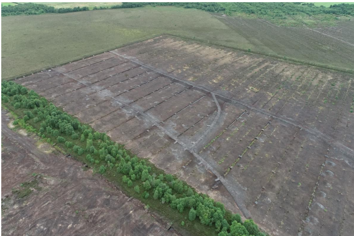
Figure 5.5 Example of cell bunding on cutover along with drain blocking with peat dams on the high bog
