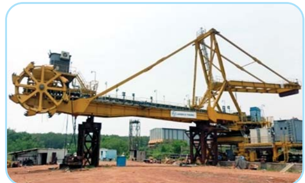
Infrastructure facilities for Road Transportation from Gangavaram Port Limited(GPL) - Wheel on Boom Reclaimer
