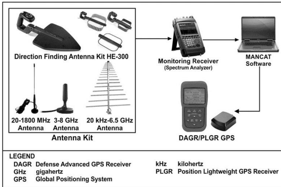
Figure C-1. S2AS and supporting equipment
