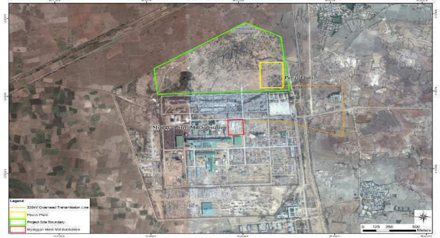
Figure 3.5 Proposed Alignment 230kV Overhead Transmission Line Route from Power Plant to Upgraded Myingyan Steel Mill sub-station [9]
