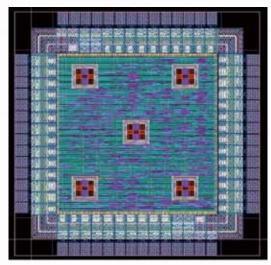
Fig. 1. Programmable fabric generated by the structure Application-Specific Integrated Circuit (ASIC) platform for adaptively LED backlight control on LCD TV.
