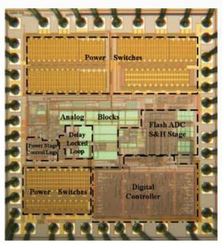
Fig. 3. Chip micrograph of Single-Inductor Triple-Output (SITO) DC-DC converter.
