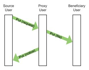
Figure 2-6: Proxy Put Operations, Sequence of Events
