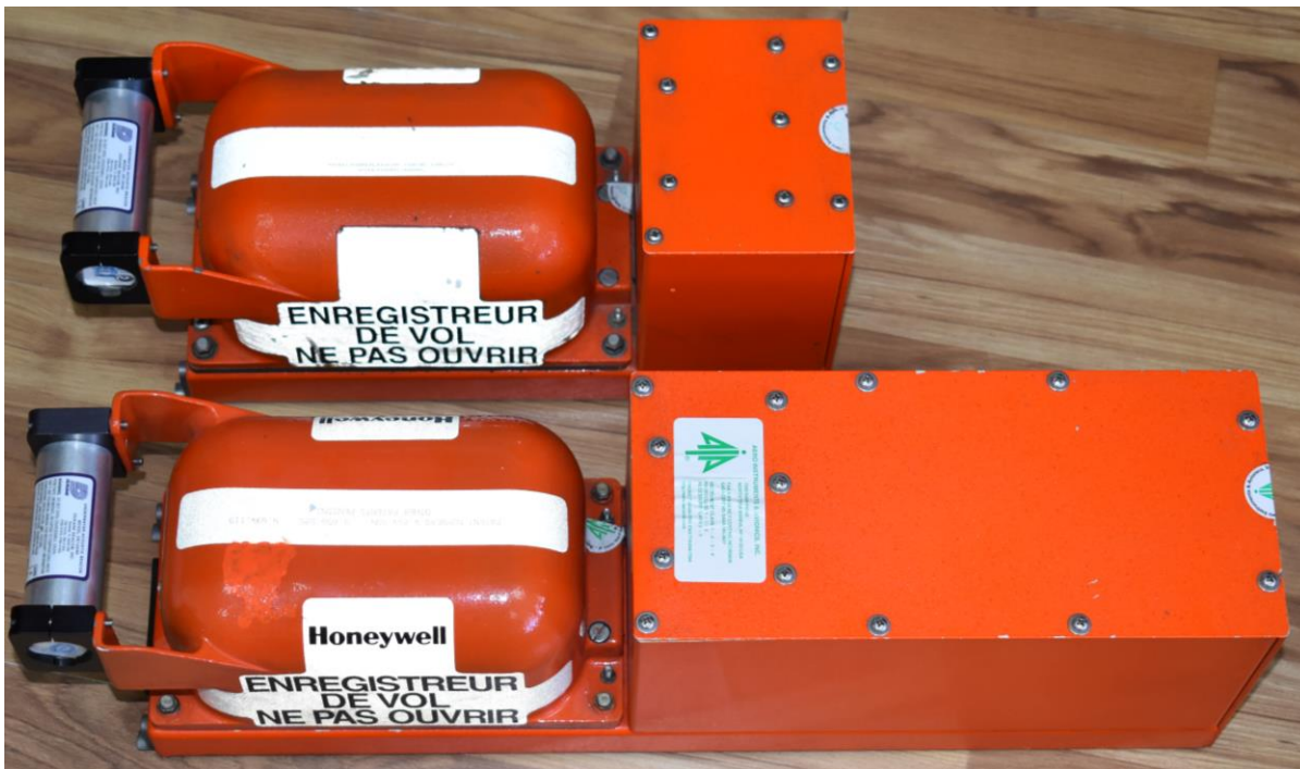
FIGURE No. 9 – A photo depicting the Cockpit Voice Recorder (upper) and Flight Data Recorder
