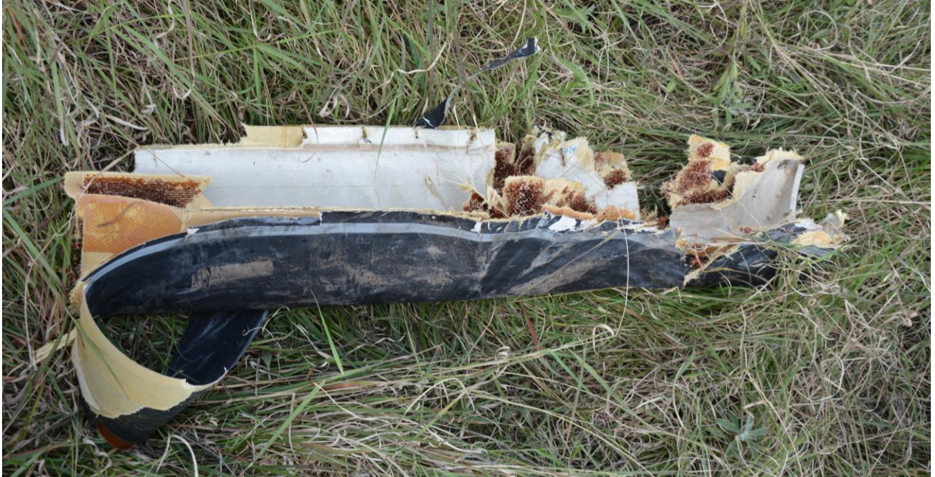
FIGURE No. 7- A photo of the right outboard horizontal stabilizer leading edge de-icing boot at the 5Y-NNJ crash site
