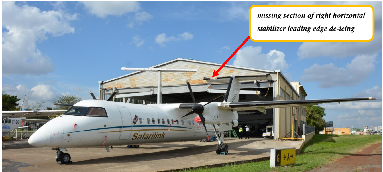
FIGURE No. 4 – A photo of 5Y-SLK parked outside the operator's hangar after the midair collision accident
