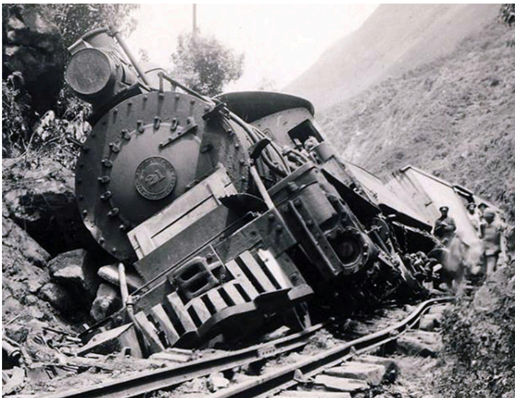
No. 21 after a derailment. The location and date are unknown but it can be seen that the loco now carries an electric headlamp but not yet replacement valve chests or knuckle coupler.
