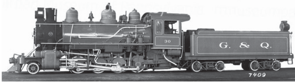
BLW image 07409-1 available from the Railroad Museum of Pennsylvania. These would appear to have been the first G&Q locos to have been supplied with piston valves, and it looks as though there is a knuckle coupler fitted too.
