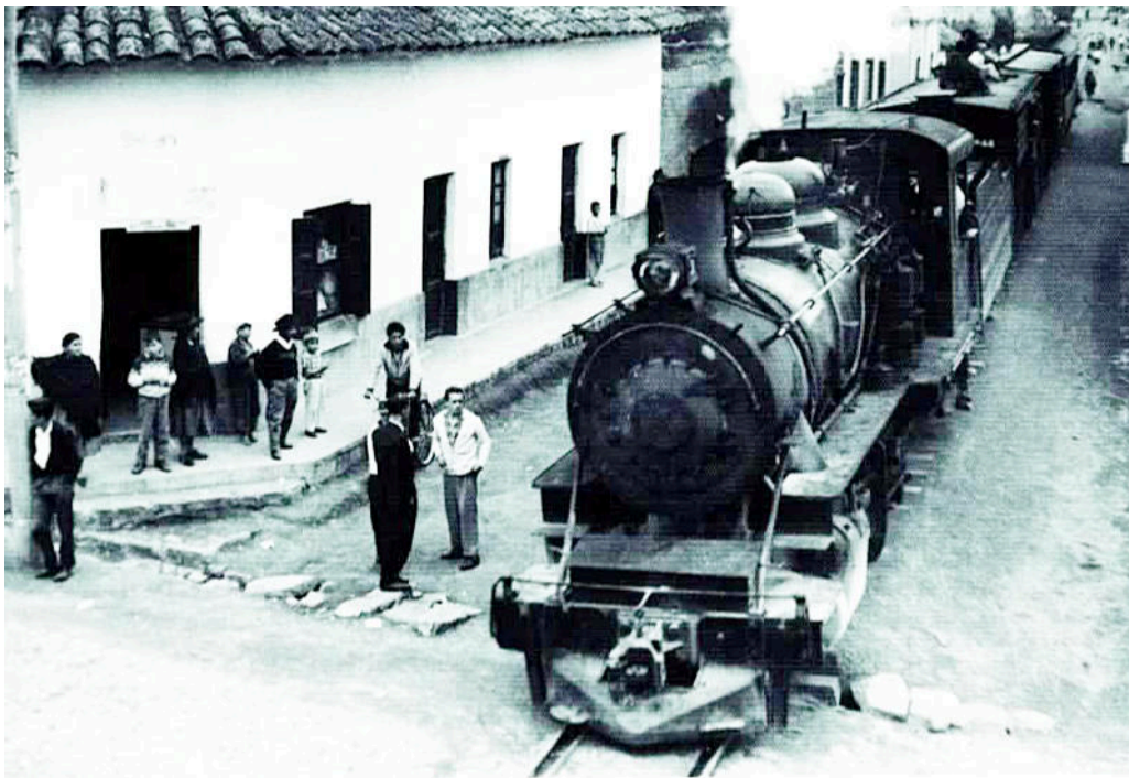
FCQE no. 3 on a short mixed train in a street, supposedly at Atuntaqui north of Ibarra. The original ribbed wooden pilot has been replaced by one of sheet steel.
