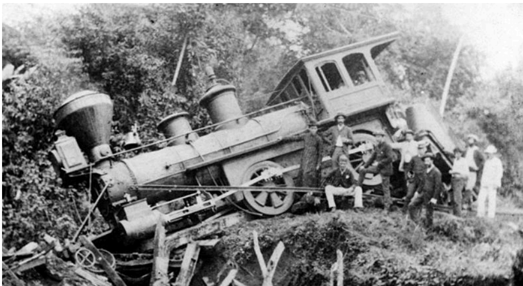
The two-part bolted-on balance weights seen on the driving wheels here were certainly a Baldwin feature during the 1870s.
