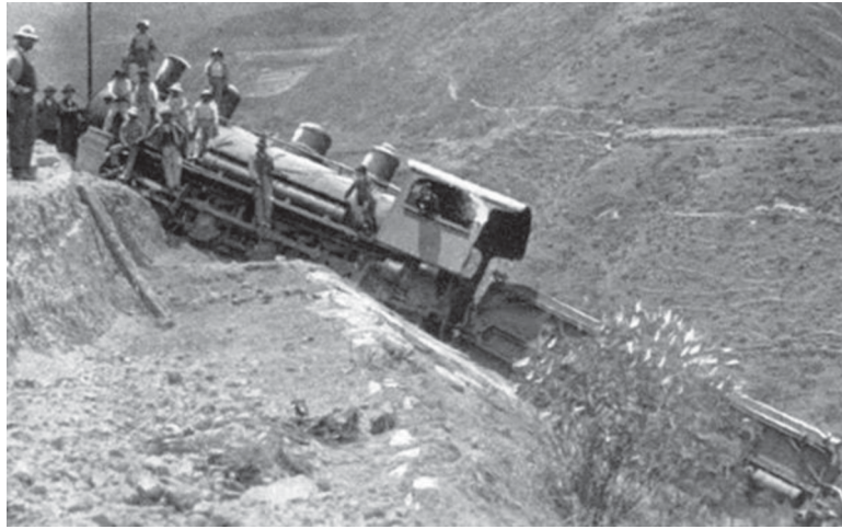
An accident to one of the Vaucrain-cylindered locos, as shown in the Baldwin Magazine during the 1920s. This image may well have been reversed for publication, unless the air reservoir on one or more of these engines had been moved to the right hand side. However, it has been reversed again here.
