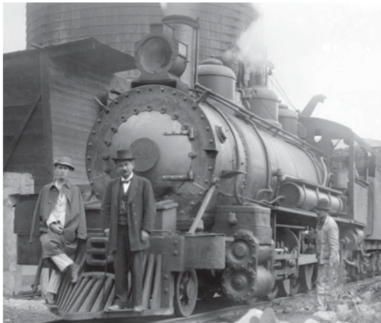
Vaucrain 2-8-0 no. 23 in about 1920, having lost both its chimney cap and the lagging around its cylinders.
