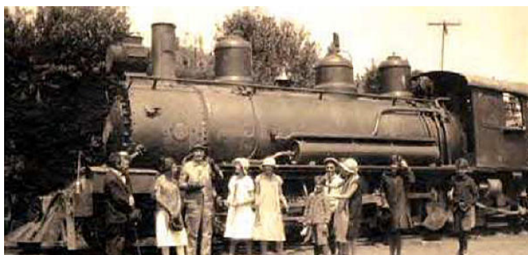
A view of the left hand side of one of the Vaucrain locos, after a turbo-generator had been installed immediately in front of the cab. Note that the chimney has been shortened but the sand-domes seem to be taller than those seen in the builders' photo above.
