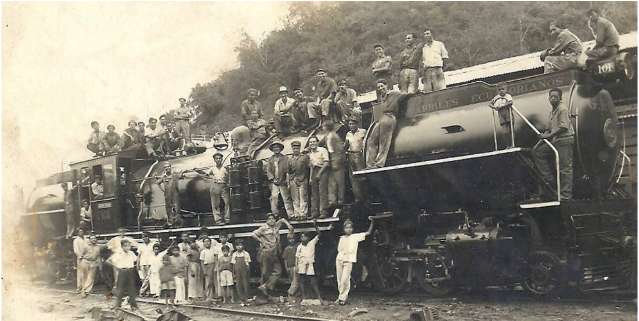
Two unattributed photos provided by courtesy of the late Gavin Hamilton show how the Garratts were rebuilt with cylindrical tank and bunker aligned to the boiler in Algerian style. 'FERROCARRILES EQUATORIANOS' is painted along the vertical plates at the top of the tank, and 'G. & Q.' across the circular front. It also would appear that this engine has a round-topped firebox, and it may therefore have been no. 101 after its explosion in 1933.
