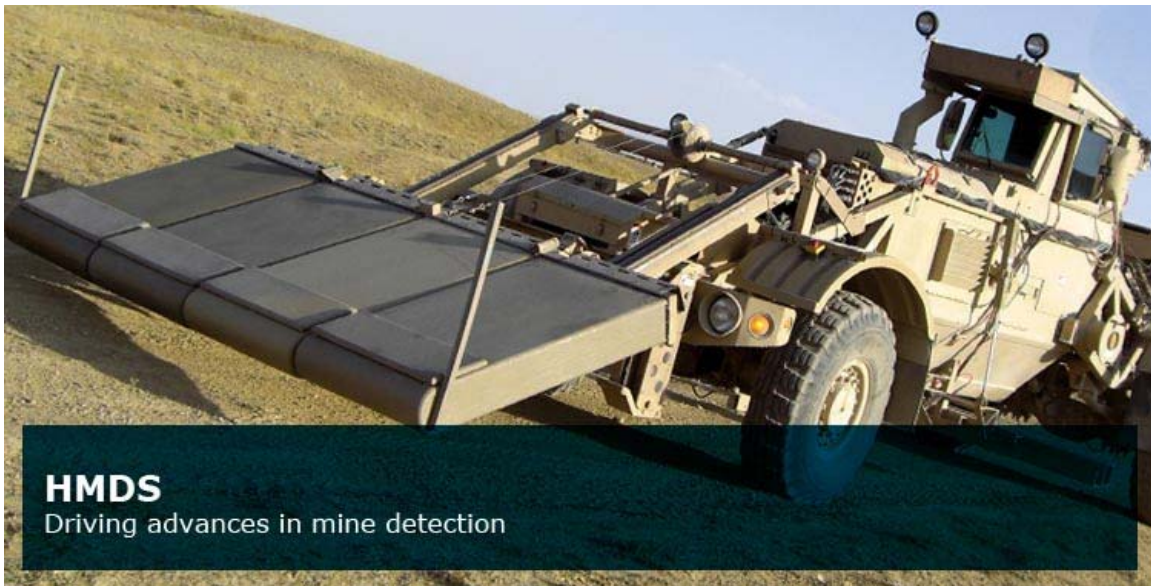
Figure 5-1. HMDS in field.
