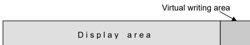
Figure 4-15 Display area of one line lateral direction scrolling and the virtual writing area
