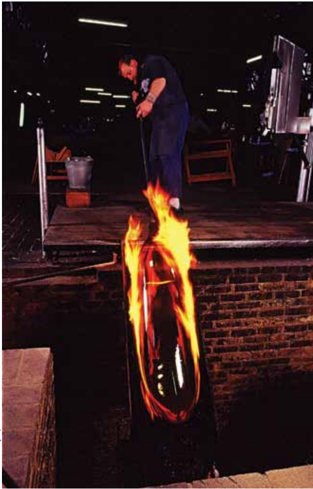
Utilizing the centuries-old mouth-blown technique, a Lamberts craftsman works a large balloon of molten glass to create a sheet of Lamberts 'new antique' glass.
