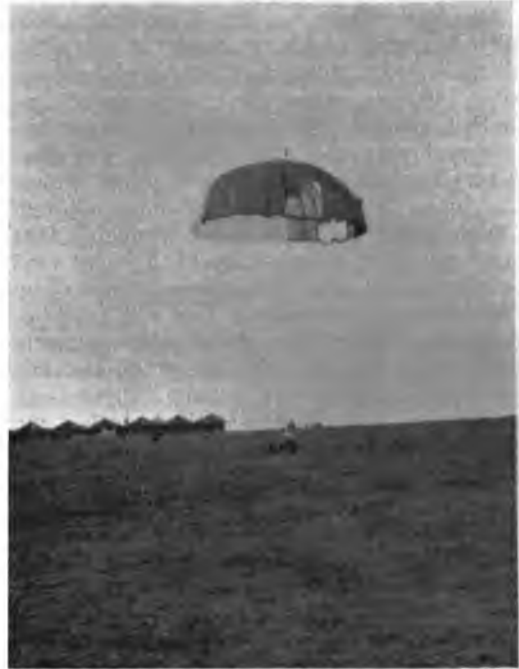
The moment of joy. The 'L' shaped modifications which give the parachute its forward motion can be clearly seen.
