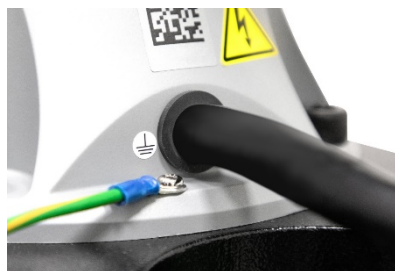
Figure 24: Securing the ground wire with the robot
