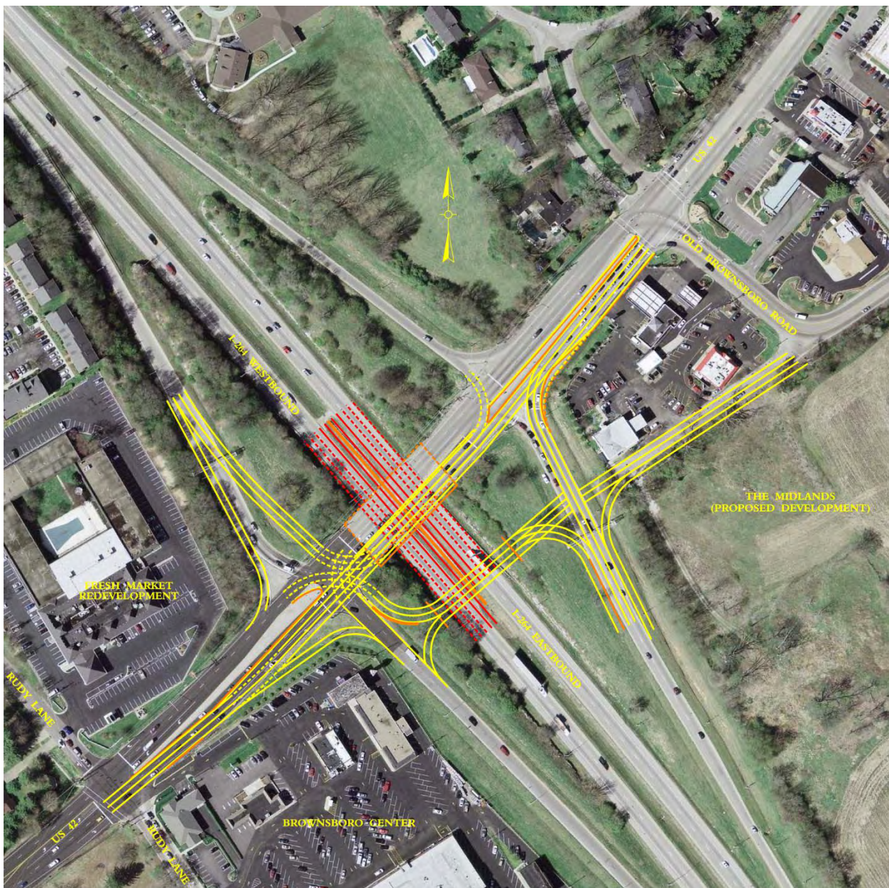
Figure 13 Initial Alternative 4: Split Diamond Interchange (SDI)
