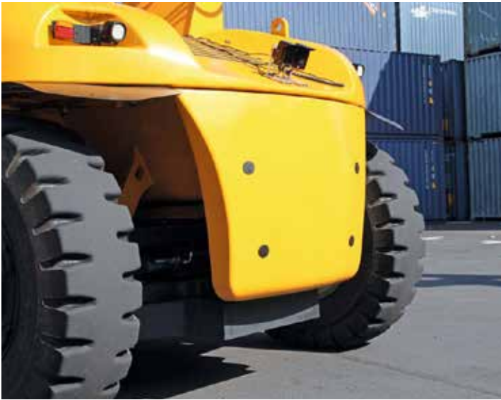
Automatic collision avoidance: 3D camera at the rear automatically warns of obstacles and possible collisions.
