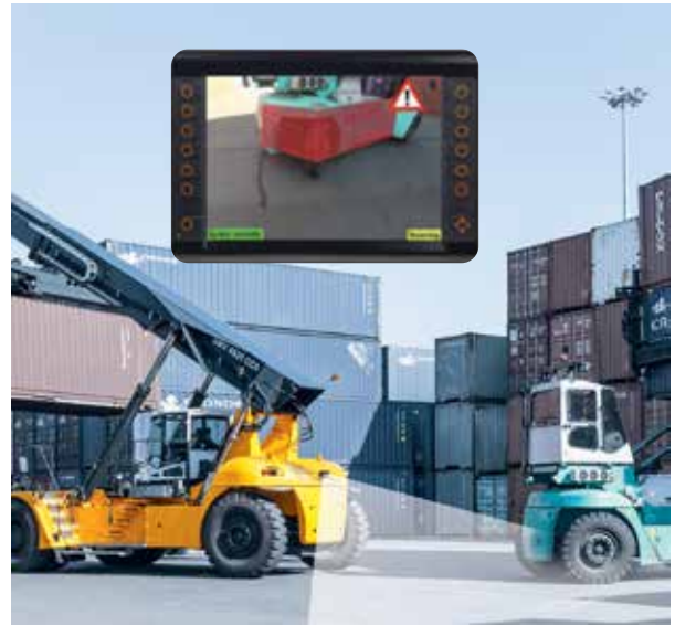
Automatic collision avoidance: 3D camera at the rear automatically warns of obstacles and possible collisions.
