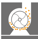
Pump Eccentricity, cavitation
