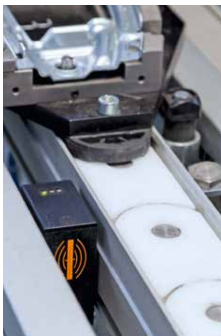
The ID tag chip is installed at the base of the workpiece carrier. The chip can store up to 224 bits.
