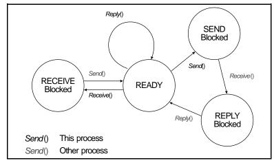
Figure 2. States involved in a typical send-receive-reply transaction.
