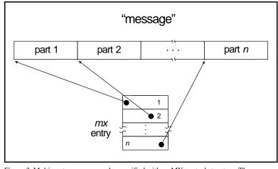
Figure 3. Multi-part messages can be specified with an MX control structure. The microkernel assembles these into a single data stream.
