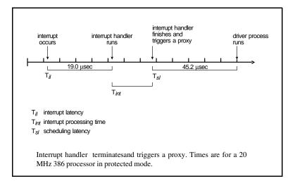
The interrupt latency  $(T_{i})$  in the above diagram represents the minimum latency—that which occurs when interrupts were fully enabled at the time the interrupt occurred. Worst-case interrupt latency will be this time plus the longest time in which QNX, or the running QNX process, disables CPU interrupts.
